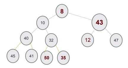
To fix the heap property on a delete BUBBLE DOWN! Worst case: O(logN)
