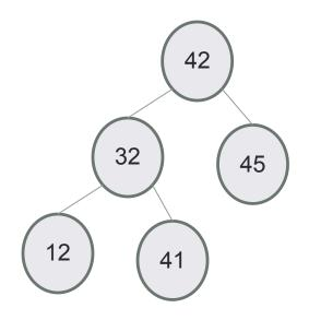
*Height of a node:* the height of a node is the number of edges on the longest path from the node to a leaf *Height of a tree:* the height of the root of the tree Height of this tree is 2.
